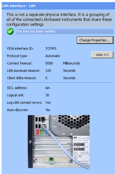
Figure 8 LAN Interface Properties Pane
